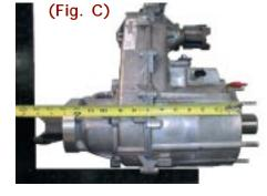
Since the Atlas is 3.0" shorter than your stock transfer case, your rear driveshaft would then need to be lengthened 3.0". This difference is now added to the measurement taken from your stock driveline, as recommended in the Preparation section. You would now have your new rear driveshaft length.
