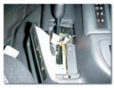
The stock console will require disassembly and the stock transfer case linkage will need to be removed.
