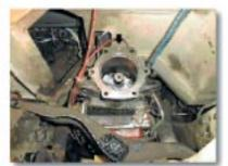
The stock Bronco Dana 20 transfer case is normally indexed onto the stock adapter housing with an aluminum bearing retainer. When using the Atlas, this
