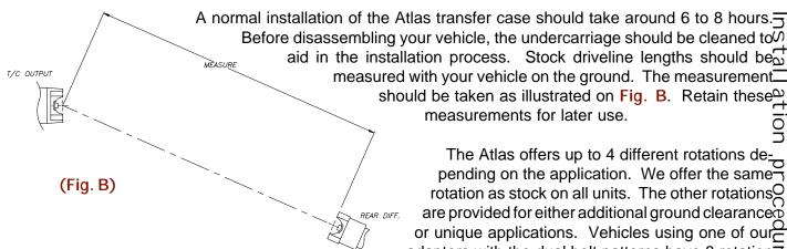
aid in the installation process. Stock driveline lengths should be of measured with your vehicle on the ground. The measurement should be taken as illustrated on Fig. B. Retain these<sup>20</sup>, measurements for later use.
