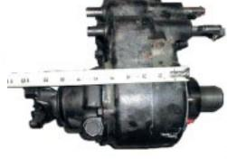
The stock Dana 20 transfer case measured 10-1/4" from the surface of the stock adapter housing to the face of the output yoke.
