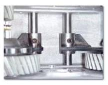
Using a plastic dead blow hammer, use one hand to support the Atlas shift forks inside the case to prevent binding on the shift rails and the other hand on the hammer *lightly* tapping the shift rails from the front of the case. This provides an easy way of pulling the shifter control from the Atlas case. Once the shift control is removed, clean both the case and shifter control mating surfaces.
