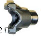
NOTE: If you replace the front 26 spline yoke with any of the yokes above, the nut that retains the yoke has a torque specification of 130-135 ft./lbs. When replacing the front or rear 32 spline yoke with any of the yokes listed above, the nut that retains the yoke has a torque specifications of 150-155 ft./lbs.
