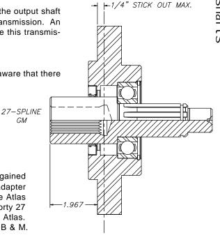
700R & 4L60 4WD: When obtaining a 700R or 4L60 out of a 4WD vehicle, the output shaft should have a stickout length of 2.75" from the rear square flange of the transmission. Adapter housing P/N AS-9111 (2.5" long) can be purchased from us to use these transmissions with this stock 27 spline 4WD output shaft.
