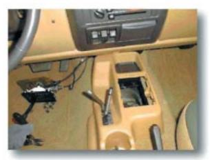
Place the stock console in its original position to test fit the Atlas handles. Rotate the twin stick assembly so that it aligns with the console slot. Once the correct position is obtained, remove the console again.
