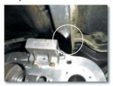
Upper body modification for clearance when the Atlas is rotated shallower than stock.
