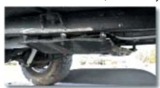
Skid pan with spacers. Spacers can usually be eliminated with the shallow transfer case rotation and minimal transmission mount height.
