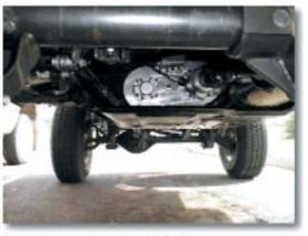
Note the new Atlas installed with no crossmember spacers (which robs you of precious ground clearance), and the gain of over 6 inches of new and much needed REAR driveshaft length.
