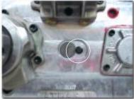
you will need to remove the cluster pin bolts from both the front and rear of the transfer case (photos
