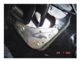
The sticks will come up through the stock floorboard hole. You will be required to cover a small portion of the stock hole. The rear driver's side will need a piece of sheet metal to be added. Make sure the handles move freely and don't touch the floorboard. Interference will cause the unit to pop out of gear.
