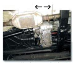
Because of the shorter overall design, the Atlas tucks up behind the crossmember. It reduces the high center problems on longer wheelbase vehicles.
